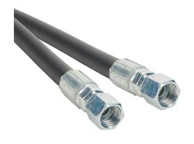
Gates ProFlex petroleum based hydraulic fluid hose assembly, synthetic rubber, braided steel wire reinforced, black, 1/2in inside diameter, 0.81in outside diameter, (2) -8 female straight JIC 37 deg fittings, 4ft working length.
