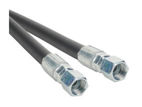
Gates ProFlex petroleum based hydraulic fluid hose assembly, synthetic rubber, braided steel wire reinforced, black, 1/2in inside diameter, 0.81in outside diameter, (2) -8 female straight JIC 37 deg fittings, 2ft working length.
