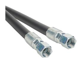
Gates ProFlex petroleum based hydraulic fluid hose assembly, synthetic rubber, braided steel wire reinforced, black, 1/2in inside diameter, 0.81in outside diameter, (2) -8 female straight JIC 37 deg fittings, 10ft working length.
