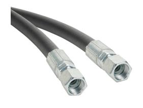
Gates MXT petroleum based hydraulic fluid hose assembly, synthetic rubber, braided steel wire reinforced, black, 1/2in inside diameter, 0.795in outside diameter, (2) -8 female straight JIC 37 deg fittings, 8ft working length.
