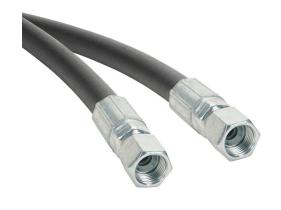
Gates MXT petroleum based hydraulic fluid hose assembly, synthetic rubber, braided steel wire reinforced, black, 1/2in inside diameter, 0.795in outside diameter, (2) -8 female straight JIC 37 deg fittings, 6ft working length.
