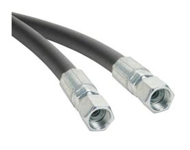
Gates MXT petroleum based hydraulic fluid hose assembly, synthetic rubber, braided steel wire reinforced, black, 1/2in inside diameter, 0.795in outside diameter, (2) -8 female straight JIC 37 deg fittings, 4ft working length.
