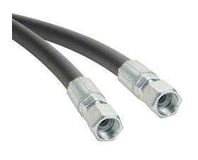
Gates MXT petroleum based hydraulic fluid hose assembly, synthetic rubber, braided steel wire reinforced, black, 1/2in inside diameter, 0.795in outside diameter, (2) -8 female straight JIC 37 deg fittings, 2ft working length.
