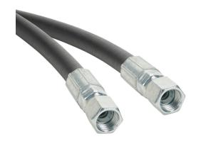
Gates MXT petroleum based hydraulic fluid hose assembly, synthetic rubber, braided steel wire reinforced, black, 1/2in inside diameter, 0.795in outside diameter, (2) -8 female straight JIC 37 deg fittings, 10ft working length.
