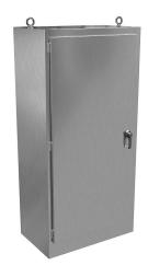
Hammond disconnect enclosure, NEMA 3R/4/4X/12/13, right flange, 84 x 41 x 24in (HxWxD), freestanding, 304 stainless steel, #4 brush finish, single-door, 3-point padlocking handle.
