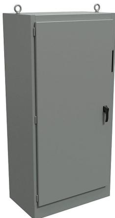
Hammond disconnect enclosure, NEMA 12, right flange, 84 x 41 x 24in (HxWxD), freestanding, carbon steel, ANSI 61 gray, powder coat finish, single-door, 3-point padlocking handle.
