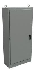
Hammond disconnect enclosure, NEMA 12, right flange, 84 x 41 x 18in (HxWxD), freestanding, carbon steel, ANSI 61 gray, powder coat finish, single-door, 3-point padlocking handle.
