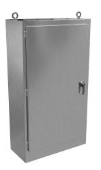
Hammond disconnect enclosure, NEMA 3R/4/4X/12/13, right flange, 72 x 41 x 18in (HxWxD), freestanding, 304 stainless steel, #4 brush finish, single-door, 3-point padlocking handle.
