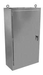
Hammond disconnect enclosure, NEMA 3R/4/4X/12/13, right flange, 72 x 41 x 18in (HxWxD), freestanding, 304 stainless steel, #4 brush finish, single-door, 3-point padlocking handle.
