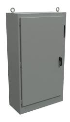
Hammond disconnect enclosure, NEMA 12, right flange, 72 x 41 x 18in (HxWxD), freestanding, carbon steel, ANSI 61 gray, powder coat finish, single-door, 3-point padlocking handle.
