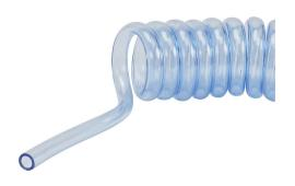
NITRA pneumatic coiled tubing, ether-based polyurethane, clear blue, 5/32in (4mm) outside diameter, 0.093in inside diameter, 40 coils, 5.5ft (1.68m) working length.
