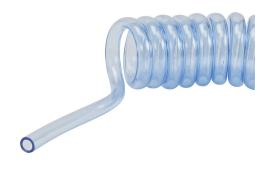
NITRA pneumatic coiled tubing, ether-based polyurethane, clear blue, 5/32in (4mm) outside diameter, 0.093in inside diameter, 20 coils, 3.9ft (1.19m) working length.
