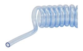
NITRA pneumatic coiled tubing, ether-based polyurethane, clear blue, 1/4in outside diameter, 0.156in inside diameter, 20 coils, 5.8ft (1.77m) working length.
