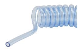
NITRA pneumatic coiled tubing, ether-based polyurethane, clear blue, 5/16in (8mm) outside diameter, 5mm inside diameter, 40 coils, 8.8ft (2.68m) working length.
