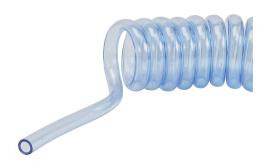
NITRA pneumatic coiled tubing, ether-based polyurethane, clear blue, 5/16in (8mm) outside diameter, 5mm inside diameter, 10 coils, 3.3ft (1.01m) working length.
