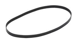
SureMotion timing belt, 0.08in MXL pitch, 1/4in wide, 195 tooth, 15.6in pitch length (circumference), polyurethane, polyester reinforced. Package of 3.
