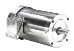
Leeson Washguard SST Duck premium efficiency AC induction motor, washdown and inverter rated, 2hp, 3-phase, 208-230/460 VAC, 1800rpm, TEFC, NEMA 145TC frame, stainless steel, C-face mount.
