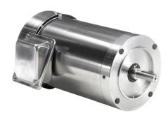
Leeson Washguard SST Duck premium efficiency AC induction motor, washdown and inverter rated, 2hp, 3-phase, 208-230/460 VAC, 1800rpm, TEFC, NEMA 56C frame, stainless steel, C-face mount.
