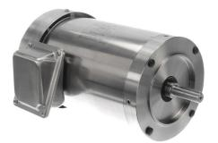
Leeson Washguard SST Duck premium efficiency AC induction motor, washdown and inverter rated, 1hp, 3-phase, 208-230/460 VAC, 1800rpm, TEFC, NEMA 56C frame, stainless steel, C-face mount.
