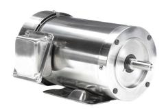
Leeson Washguard SST Duck premium efficiency AC induction motor, washdown and inverter rated, 2hp, 3-phase, 208-230/460 VAC, 1800rpm, TEFC, 56HC frame, stainless steel, Cface/rigid base mount.
