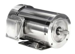
Leeson Washguard SST Duck premium efficiency AC induction motor, washdown and inverter rated, 1-1/2hp, 3-phase, 208-230/460 VAC, 1800rpm, TEFC, NEMA 56HC frame, stainless steel, C-face/rigid base mount.
