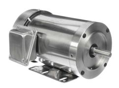
Leeson Washguard SST Duck premium efficiency AC induction motor, washdown and inverter rated, 1-1/2hp, 3-phase, 208-230/460 VAC, 3600rpm, TEFC, NEMA 56HC frame, stainless steel, C-face/rigid base mount.
