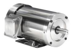
Leeson Washguard SST Duck premium efficiency AC induction motor, washdown and inverter rated, 2hp, 3-phase, 208-230/460 VAC, 1800rpm, TEFC, NEMA 145TC frame, stainless steel, C-face/rigid base mount.
