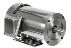
Leeson Washguard SST Duck premium efficiency AC induction motor, washdown and inverter rated, 2hp, 3-phase, 208-230/460 VAC, 3600rpm, TEFC, NEMA 145TC frame, stainless steel, C-face/rigid base mount.
