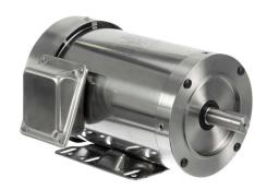
Leeson Washguard SST Duck premium efficiency AC induction motor, washdown and inverter rated, 2hp, 3-phase, 208-230/460 VAC, 3600rpm, TEFC, 145TC frame, stainless steel, C-face/rigid base mount.
