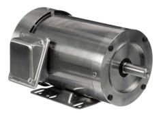
Leeson Washguard SST Duck premium efficiency AC induction motor, washdown and inverter rated, 1hp, 3-phase, 208-230/460 VAC, 1800rpm, TEFC, 143TC frame, stainless steel, Cface/rigid base mount.
