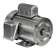
Leeson Washguard SST Duck standard efficiency AC induction motor, washdown, 1hp, 1-phase, 115/230 VAC, 1800rpm, TEFC, NEMA 56C frame, stainless steel, C-face/rigid base mount.
