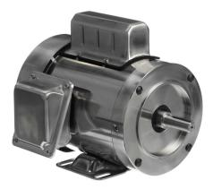
Leeson Washguard SST Duck premium efficiency AC induction motor, washdown, 3/4hp, 1-phase, 115/230 VAC, 1800rpm, TEFC, NEMA 56C frame, stainless steel, C-face/rigid base mount.
