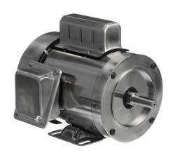
Leeson Washguard SST Duck premium efficiency AC induction motor, washdown, 3/4hp, 1-phase, 115/230 VAC, 1800rpm, TEFC, 56C frame, stainless steel, C-face/rigid base mount.
