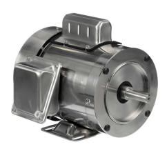
Leeson Washguard SST Duck standard efficiency AC induction motor, washdown, 1/2hp, 1-phase, 115/230 VAC, 1800rpm, TEFC, 56C frame, stainless steel, C-face/rigid base mount.
