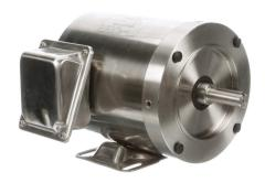
Leeson Washguard SST Duck premium efficiency AC induction motor, washdown and high-performance inverter duty, 3/4hp, 3-phase, 208-230/460 VAC, 1800rpm, TENV, 56C frame, stainless steel, C-face/rigid base mount.
