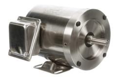
Leeson Washguard SST Duck premium efficiency AC induction motor, washdown and high-performance inverter duty, 3/4hp, 3-phase, 208-230/460 VAC, 1800rpm, TENV, NEMA 56C frame, stainless steel, C-face/rigid base mount.
