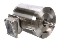
Leeson Washguard SST Duck premium efficiency AC induction motor, washdown and high-performance inverter duty, 1/2hp, 3-phase, 208-230/460 VAC, 1800rpm, TENV, NEMA 56C frame, stainless steel, C-face mount.
