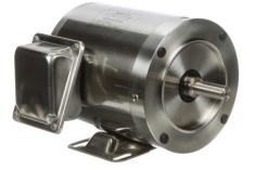
Leeson Washguard SST Duck premium efficiency AC induction motor, washdown and high-performance inverter duty, 1/2hp, 3-phase, 208-230/460 VAC, 1800rpm, TENV, NEMA 56C frame, stainless steel, C-face/rigid base mount.
