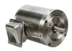
Leeson Washguard SST Duck premium efficiency AC induction motor, washdown and high-performance inverter duty, 1/3hp, 3-phase, 208-230/460 VAC, 1800rpm, TENV, NEMA 56C frame, stainless steel, C-face mount.
