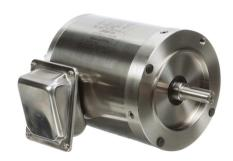
Leeson Washguard SST Duck premium efficiency AC induction motor, washdown and high-performance inverter duty, 1/3hp, 3-phase, 208-230/460 VAC, 1800rpm, TENV, 56C frame, stainless steel, C-face mount.
