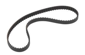
SureMotion timing belt, 1/5in XL pitch, 3/8in wide, 95 tooth, 19in pitch length (circumference), neoprene, fiberglass reinforced.
