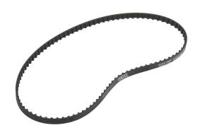
SureMotion timing belt, 1/5in XL pitch, 1/4in wide, 95 tooth, 19in pitch length (circumference), neoprene, fiberglass reinforced.
