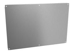
Hammond subpanel, 316 stainless steel, #4 brush finish. For use with 30x42 and 42x30 (HxW) 1418xxxx, 1422R10, 1447Sxxxx, C3R423012HCR, HW423010xxHK, and HN4WM304210xx enclosures.
