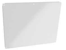
Hammond subpanel, carbon steel, RAL 9003 white, powder coat finish. For use with 36x30 (HxW) 1418xxxx, 1447Sxxxx, C3R363012HCR, and HW3630xxxxHK enclosures.
