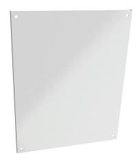
Hammond subpanel, carbon steel, RAL 9003 white, powder coat finish. For use with 24x30 and 30x24 (HxW) 1418xxxx, 1447Sxxxx, C3R3024xxHCR, and HWxxxxxxHK enclosures.
