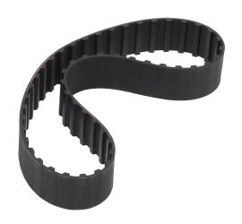
SureMotion timing belt, 3/8in L pitch, 1in wide, 50 tooth, 18.8in pitch length (circumference), neoprene, fiberglass reinforced.
