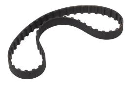
SureMotion timing belt, 3/8in L pitch, 1/2in wide, 50 tooth, 18.8in pitch length (circumference), neoprene, fiberglass reinforced.
