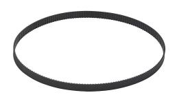
SureMotion timing belt, 0.08in MXL pitch, 1/4in wide, 184 tooth, 14.7in pitch length (circumference), neoprene, fiberglass reinforced. Package of 3.
