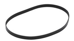
SureMotion timing belt, 0.08in MXL pitch, 1/4in wide, 180 tooth, 14.4in pitch length (circumference), polyurethane, polyester reinforced. Package of 3.
