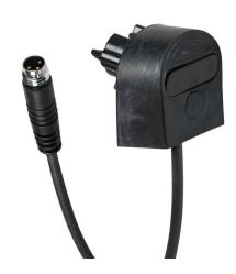
ASO Safety Solutions safety contact edge end cap, 1.6ft/0.5m cable length, 3-pin male M8. For use with 25 x 30mm safety contact edge.
