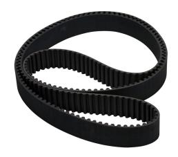
SureMotion timing belt, 8mm 8M pitch, 30mm wide, 225 tooth, 1800mm pitch length (circumference), neoprene, fiberglass reinforced.
