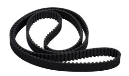
SureMotion timing belt, 8mm 8M pitch, 20mm wide, 225 tooth, 1800mm pitch length (circumference), neoprene, fiberglass reinforced.
