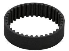
SureMotion timing belt, 5mm 5M pitch, 15mm wide, 36 tooth, 180mm pitch length (circumference), neoprene, fiberglass reinforced.
