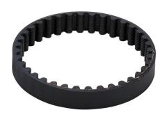
SureMotion timing belt, 5mm 5M pitch, 9mm wide, 36 tooth, 180mm pitch length (circumference), neoprene, fiberglass reinforced.
