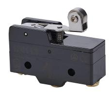
IDEM micro limit switch, lever hinge with steel roller, (1) N.O./(1) N.C. contact(s), snap action, 25.4mm hole spacing, polybutylene terephthalate, screw terminals. Package of 5.
